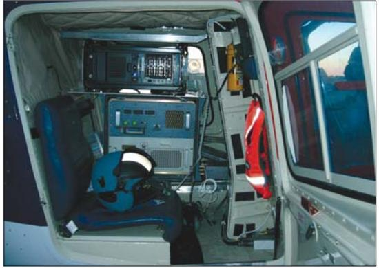
*Aerial Laser Survey equipment installed in helicopter*
